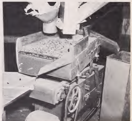
FIGURE 12.— A shaker machine used to separate stones from farmers' stock peanuts. The stones are discharged into the containers at the right and the peanuts come off the chute at the left.
